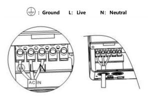
③ Properly connect the AC output wire according to the wire sequence and terminal position shown in the figure below. Please connect the ground wire first, and then the live wire and the neutral wire. The ground wire is connected to the grounding screw hole on the cabinet through the O-type terminal.
